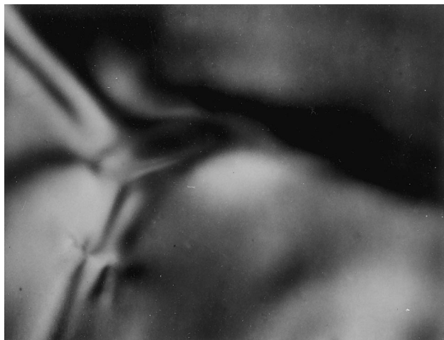
Fig. 7. Polymer 1/DDM viewed through crossed polarisers.
